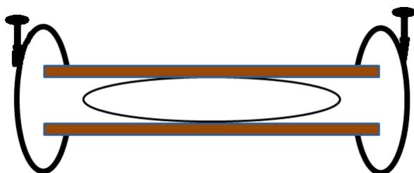
As a final note on delaminations, if you are just restoring an old board and don't plan to put it back in the water again, you can repair a delamination by forcing resin almost ready to go off between the glass and the foam through a small slit. Use C-clamps to hold two boards as shown to pressure the glass to the foam
