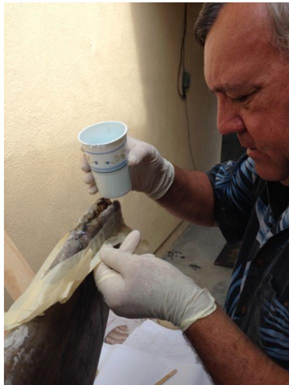
delaminated area with a layer of cloth (sometimes two layers). I generally cut a piece of 6 oz. cloth just smaller than the removed area, and squeegee it to the foam with non-finish resin. If this doesn't bring the level up enough, apply a second layer of cloth, but if you do, let it harden before applying the outer 4 oz. layer. Also, make sure you used bleached cloth. All other steps should be the same.
