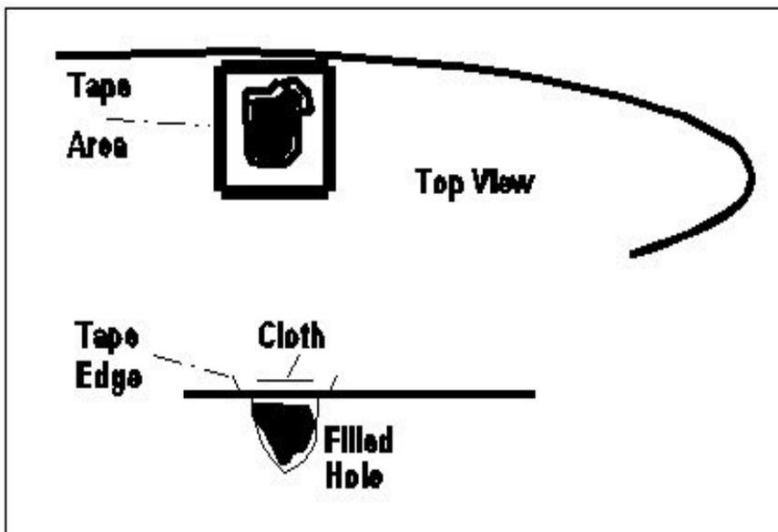
If the fracture is a stress fracture that is starting to cause a delamination or foam discoloration, use a razor blade to open the crack slightly. Let the board sit a few days to dry, and then follow the process outlined above. If the hole is large, you may need to add a little filler. Understand that repairs will not last on this type of fracture, and will need to be re-done every so often when they break open again.
